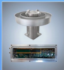
Quad-ridge "cakepan" feed and wide-band uncooled LNA
