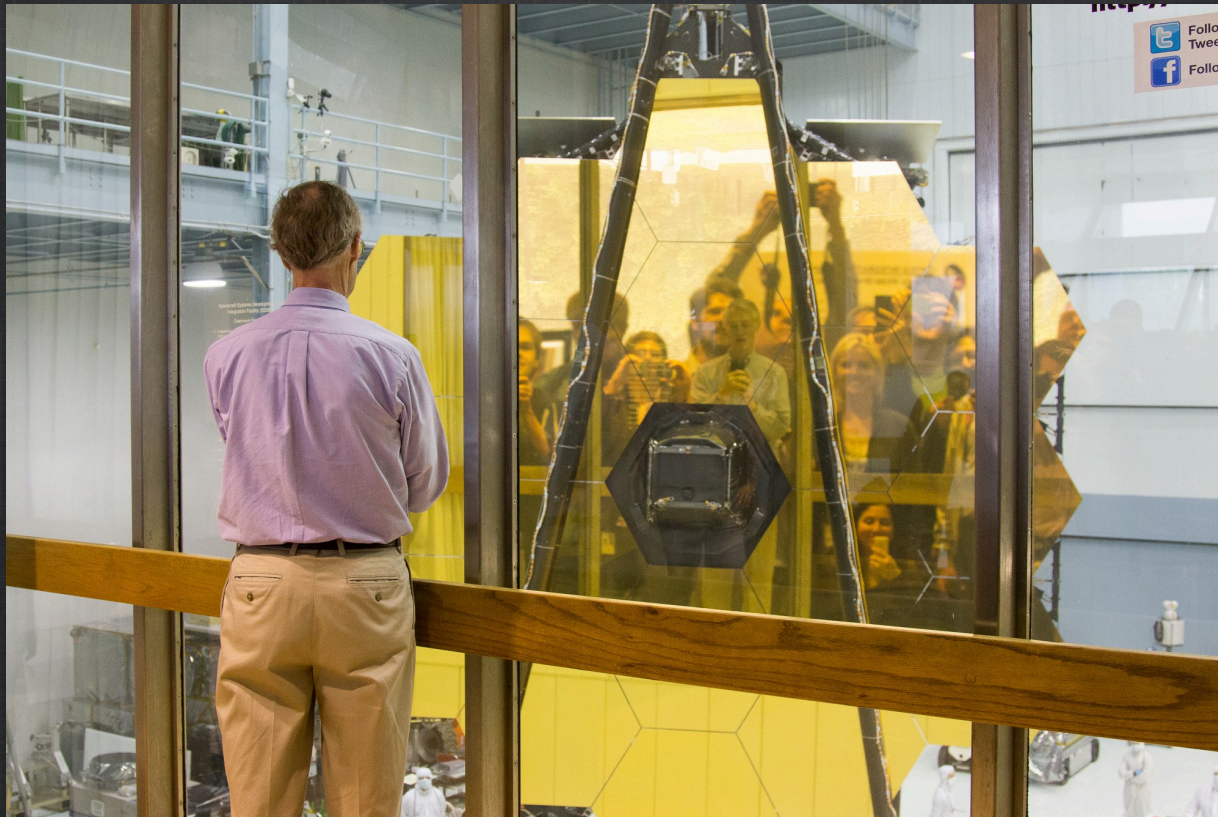
Lead project scientist John Mather admires all 18 segments of the 6.5m mirror
