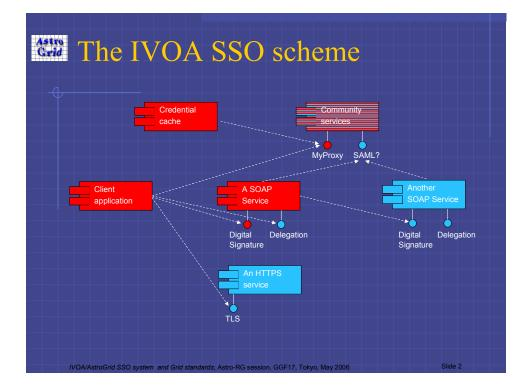
This slide shows the architecture of the IVOA single-sign-on (SSO) system adopted (and partly developed) by AstroGrid.
